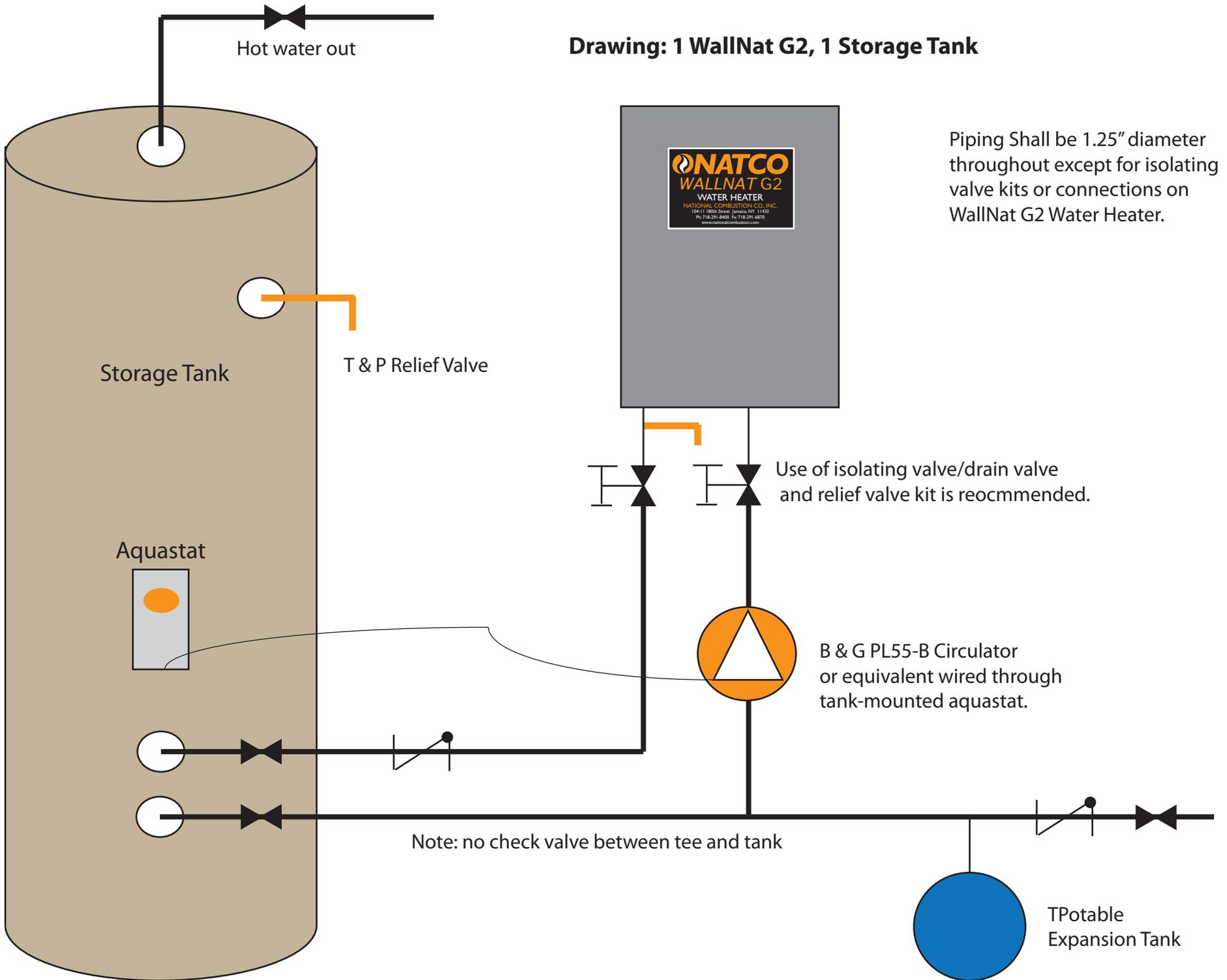
Piping Shall be 1.25" diameter throughout except for isolating valve kits or connections on WallNat G2 Water Heater.
